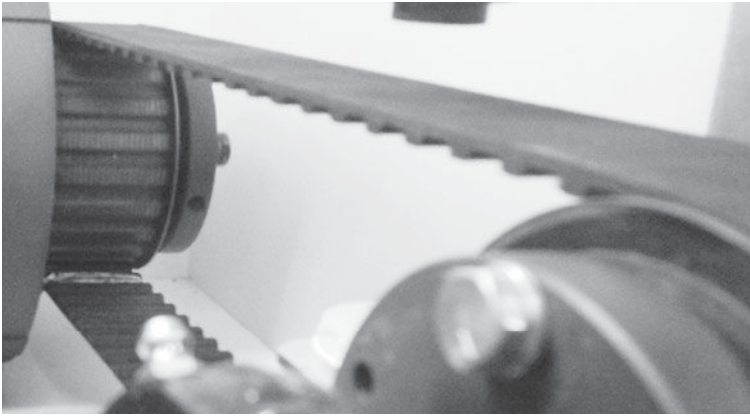
FIGURE 3.60 Positive drive (toothed) pulley and belt.
