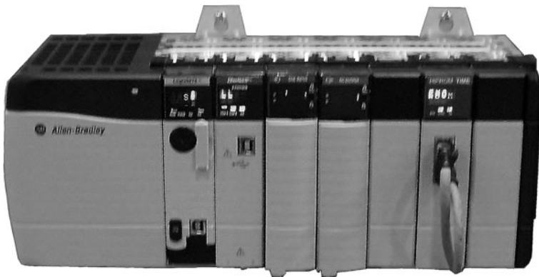
FIGURE 3.1 Allen-Bradley ControlLogix PLC.
